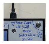
The included wide input (100...240 VAC) wall-plug power supply (HNP10l-microUSB, 5 V, 2.1 A) has to be connected to the remote control interface on the top right side (see left).
