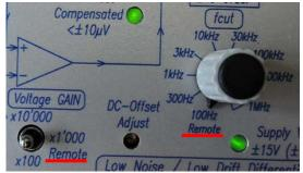
The Remote Control I/O connectors (10 pin) of the remote control interface and the LNLD Diff Amp have to be interconnected by a 1:1 cable (see below). A 4 meter long flat interconnection cable is included and it is equipped on both sides with the suitable connectors (Minitek 2x5P, 89947-710LF). Note that the plugs are
