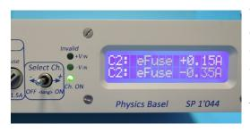
When eFuse has tripped the display shows the flashing word *eFuse* (instead of the voltage) and the two startup currents on the positive and negative voltage are shown. In the example here, the negative current of 350 mA on Channel 2 (*C2*) activates the eFuse since it is larger than the set 200 mA trip-current. Please note, that displayed currents are measured while the eFuse logic periodically restarts the
