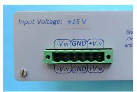
The external power supply must be able to provide the summed current of all the connected devices. Since the ten outputs can source up to  $\pm 1.5$  A the maximum total input current can be up to  $\pm 15$  A.
