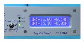
The actual input supply voltages and the total input currents, including the self-current consumption, are displayed on the local LCD. The bipolar input voltage must reach the nominal value within a tolerance of  $\pm 10\%$  before all output channels are sequentially switched ON – this prevents from a large inrush-current at power on. Note, that the positive (+Vin) and the negative (-Vin) supply
