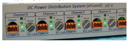
The polarity (starting from left) is the following: -5 V / GND (0 V) / +5 V
