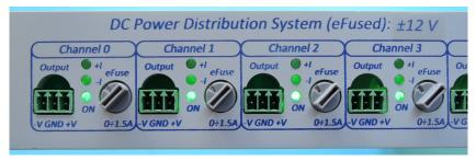
The polarity (starting from left) is the following: -12 V / GND (0 V) / +12 V
