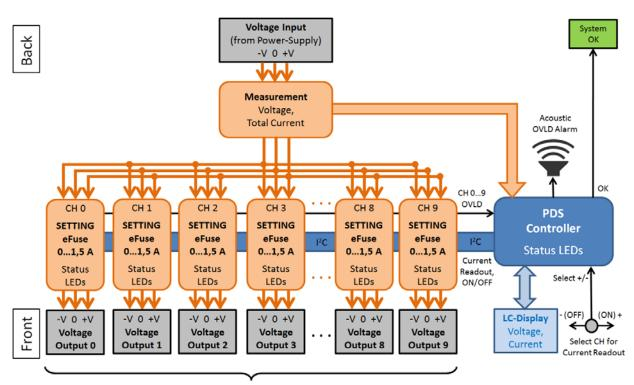
10 Voltage Outputs: ±5 V... ±18 V, eFused 0... ± 1,5 A @100 mA steps
