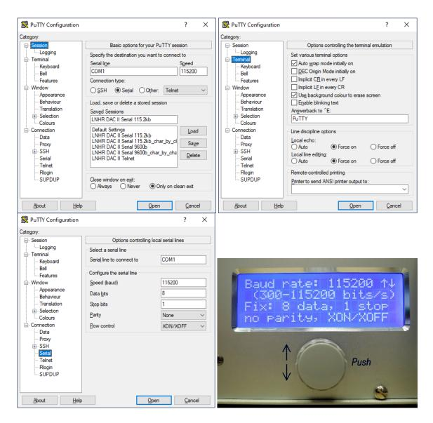
At a communication speed of 115.2 kbit/s the properties of the communication port (COM1) and its advanced settings should be like this on the host computer (Windows 10 PC):
