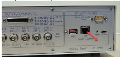
The data rate of 10 Mbps, 100 Mbps or 1 Gbps is automatically selected by the network interface card (NIC) of the host computer. The actual data rate is indicated by the right LED on the LAN port of LNHR DAC II: 10 Mbps=OFF, 100 Mbps=GREEN, 1 Gbps=YELLOW. The left LED on the LAN port shows the activity on the LAN; it is flashing when active.
