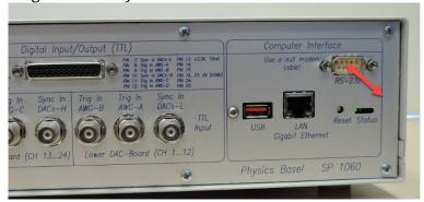
Different Baud rates from 300 to 115'200 bit/sec can be selected locally on the device under the menu item "RS-232 Settings". The following Baud rates can be selected: 300, 1200, 2400, 4800, 9600, 19200, 38400, 57600, 115200 bit/sec. At delivery the Baud rate is set to 9'600 bit/sec. Make sure that the speed of the serial port (Baud rate) on the host computer (PC) is the same as configured on the LNHR DAC II.
