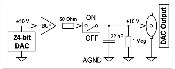
In the OFF state the output gets passively grounded (AGND) by a 1 Mega Ohm resistor in parallel with a 22 nF capacitor. The ON state is indicated on the front-panel by a LED next to the BNC connector; the color of the LED is depending on the selected bandwidth: Yellow = LBW (100 Hz) / Blue = HBW (100 kHz)
