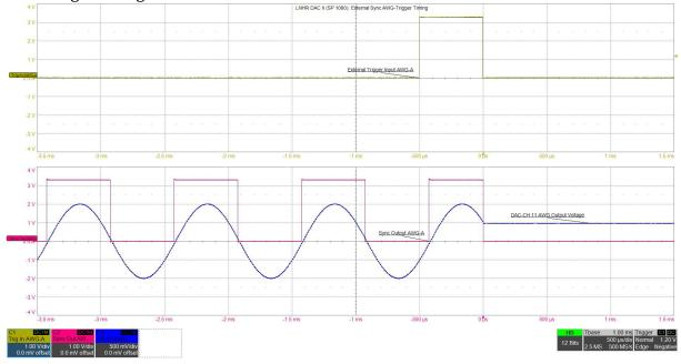
The falling-edge on the "Trig In AWG" input signal immediately stops the infinite repetitive running AWG. The rising-edge has no impact, since the AWG is already started.
