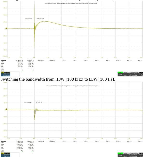
Switching the bandwidth from LBW (100 Hz) to HBW (100 kHz):
