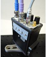
The *OIS* has a M4 thread (depth 3.5 mm) at the bottom. This allows attaching a metrical post for directly mounting the device on an optical table (see photos on the left).
