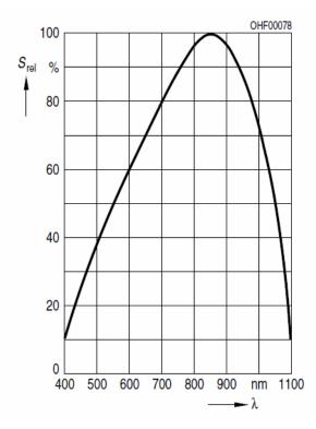
The relative spectral sensitivity of this photodiode is shown in the graph on the left; it covers a wavelength range from 400 nm to 1'100 nm. The maximal photosensitivity of 0.62 A/W (corresponds to 100%) is reached at a wavelength of 850 nm.
