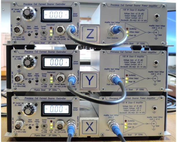
The three Power-Supplies can be easily separated from the Controllers/Amplifiers and; these are preferably arranged horizontally to allow cooling by air circulation:
