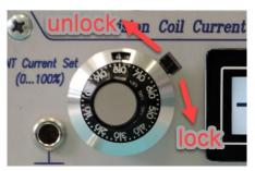
counter that displays from 0 to 9. A set value can be blocked with the black lever; this ensures that the set-point will not change due to vibration.
