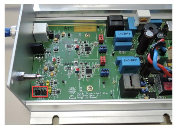
The peak-to-peak PWM-frequency dither can be selected between these values: 0% (fix 380 kHz, default), 2% (376.2...383.8 kHz), 4% (372.4... 387.6 kHz) and 8% (364.8...395.2 kHz). This dither percentage is set by the two jumpers J0 and J1 on J12:
