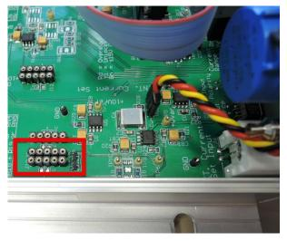
components can be installed on these two sockets; SMD (0805) components can also be soldered in. The line on the silk-layer indicates the separation of the socket:
